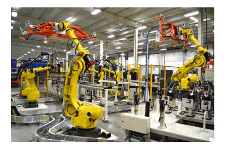
Large scale robotic system that integrates welding, dispensing, assembly, and material handling technologies to produce an automotive part.
