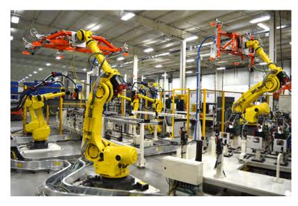
Large scale robotic system that integrates welding, dispensing, assembly, and material handling technologies to produce an automotive part.
